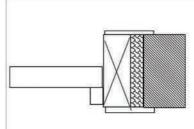
Gaps between frame and wall must be fire-stopped to the same rating as the door or as per BS 8214 using a suitable fire-stopping product.
